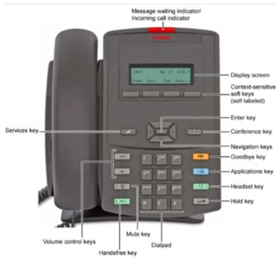
This station is basically the same as the 1110 phone, but with simpler and less expensive body, simplified button locations, four discrete direction arrows for navigation, and a number of other simplifications.
