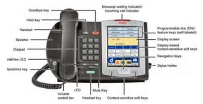
This phone is basically a 2004 phone with a touch screen for all buttons except the hold, release, mute, headset, speaker, and volume buttons. The navigation arrows were merged into a single rocker control.
