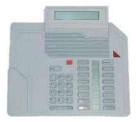
The preceding picture is of an M2216 digital phone with the optional display. If the display is present, then the top key on the right-hand button column (key 7) must be for the Program key. The Program key allows to set the display options. Note that the 2216 phone is intended for the call center environment and has a plug-in-headset that can be used for agent login and logout. Inserting or removing the headset logs in and logs out the agent at this station.
