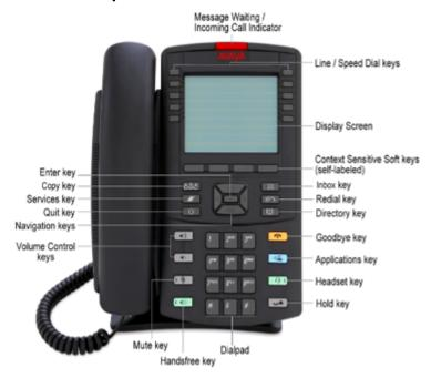
This station is somewhat of a hybrid of the 1140 and 1165 phones, with simpler and less expensive body, simplified button locations, four discrete direction arrows for navigation, and a number of other simplifications. However, it has ten programmable feature buttons, allowing up to 20 buttons to be programmed.
