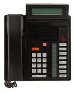
The M2008 is a multi-line telephone with eight programmable function keys. The M2008HF contains an integrated Handsfree unit.
