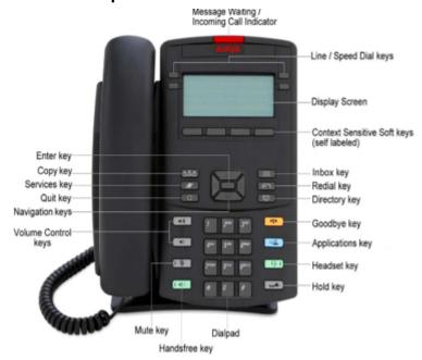
This station is basically the same as the 1120 phone, but with simpler and less expensive body, simplified button locations, four discrete direction arrows for navigation, and a number of other simplifications.
