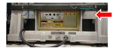
Pedestal base, with the cover removed to see the power switch and XSM in proximity
