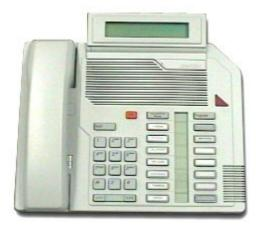
The preceding picture is of an M2616 digital phone with the optional display. If the display is present, then the top key on the right-hand button column (key 7) must be for the Program key. The Program key allows to set the display options. The 2616 phone is not intended for the call center environment, but can still be used in the call center environment.
