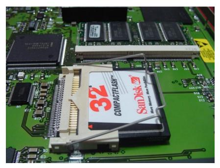
Figure 55: Position the CompactFlash in socket
