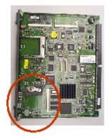
Figure 54: CompactFlash card socket on Media Card
