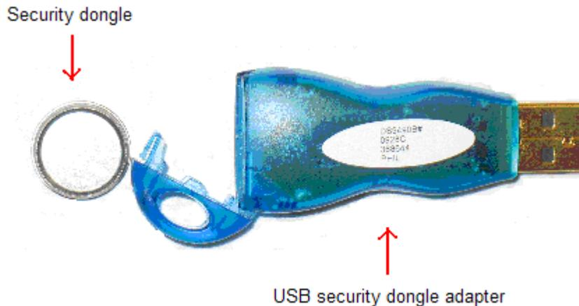
Figure 14: USB Security dongle and adapter
