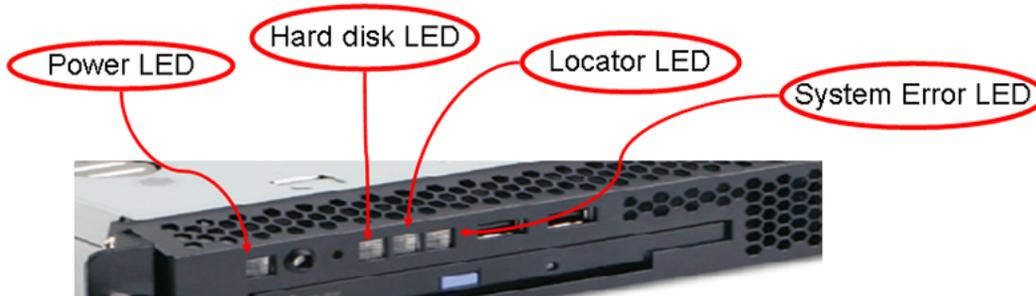
Figure 167: IBM x306m front view: LEDs
