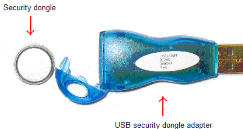
Figure 4: NTRH9220E6 USB security dongle adapter for COTS2 servers
