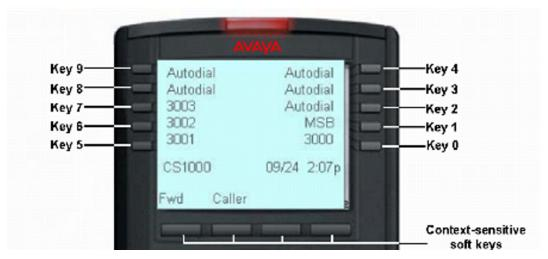
Figure 327: Programmable/DN feature keys (first page)
