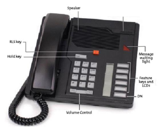
Figure 360: Meridian M2006 Digital Telephone Layout
