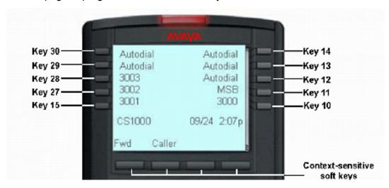
Figure 328: Programmable/DN feature keys (second page)
