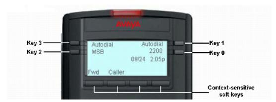
Figure 324: Avaya 1220 IP Deskphone Programmable/DN Feature keys
