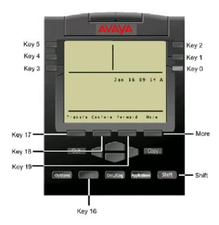
Figure 379: Avaya 3904 Digital Deskphone with feature keys 0 - 5, 16, and soft keys 17 - 19
