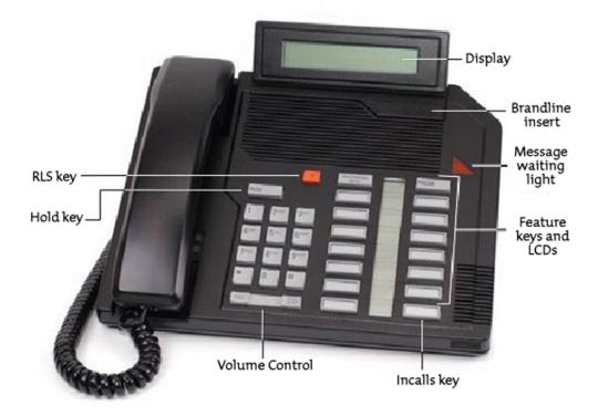
Figure 364: Meridian M2616 Digital telephone layout
