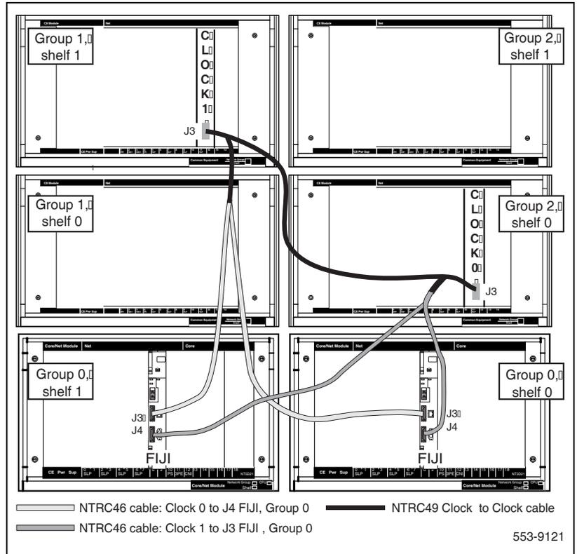
Connect the cables to the Clock Controllers as shown in Figure 103 on [page 243](#).
