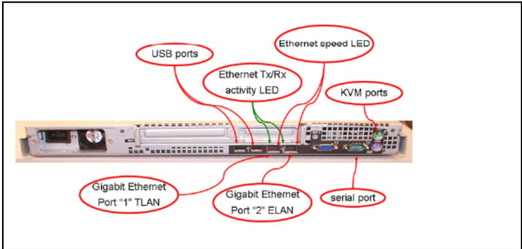
Figure 156 shows the rear view of the IBM x3350 server.
