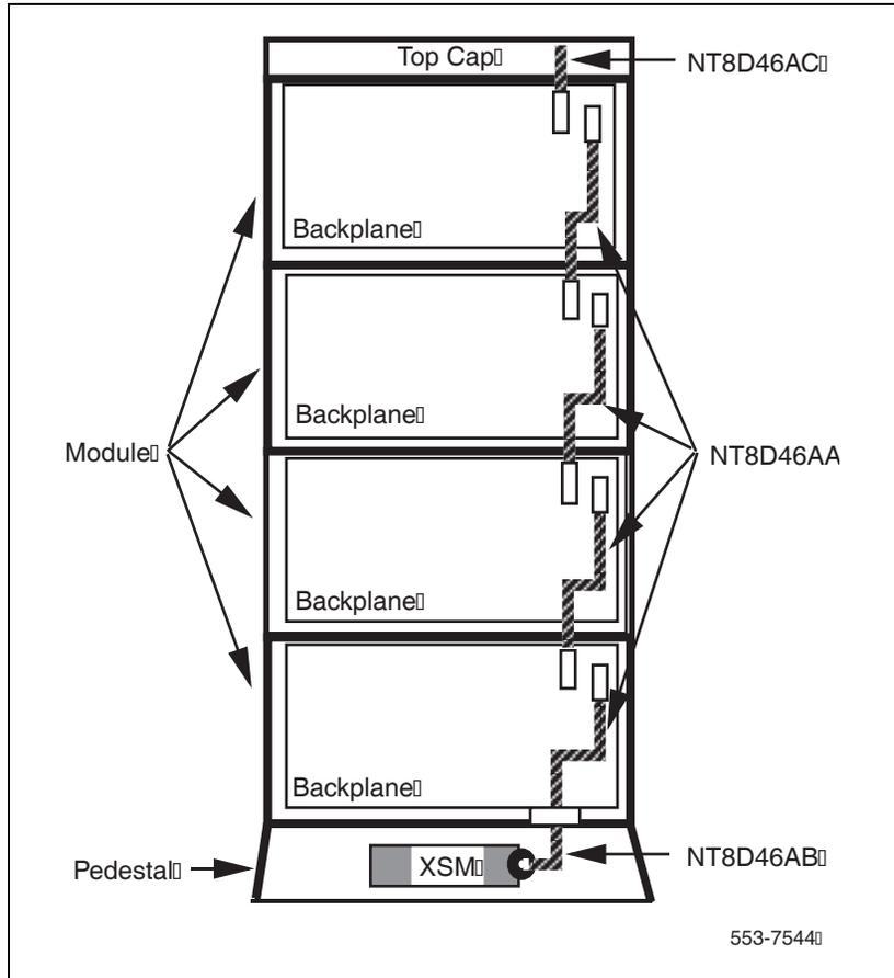
Follow the steps in Procedure 16 to cable the NT8D22 System Monitor.
