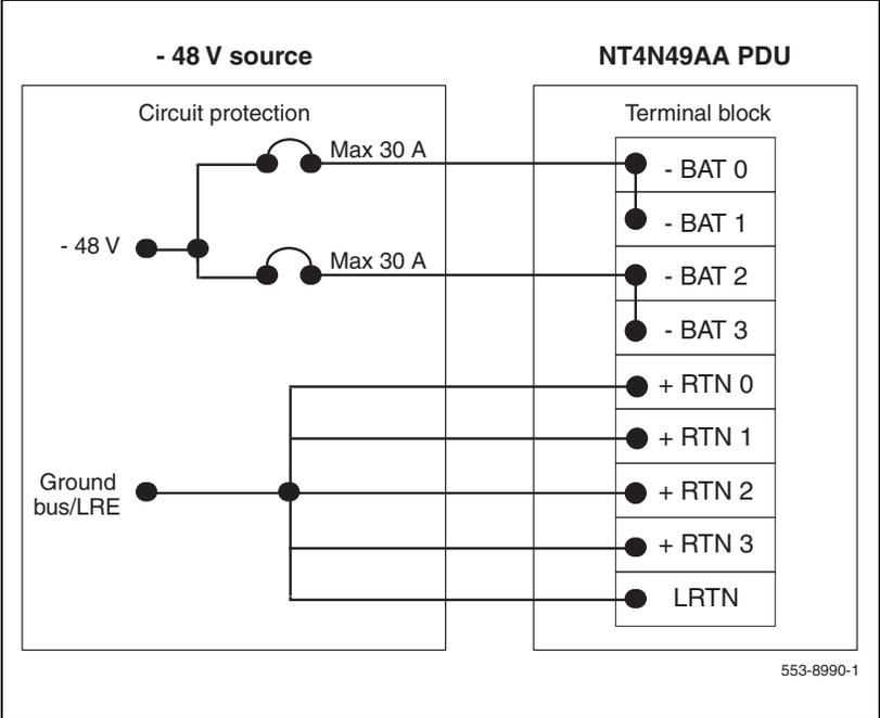
A maximum loop drop of 2 V is allowed between the pedestal, or junction box, and the external power equipment. See Table 5 for allowable wire sizes. For more information about calculating wire size, see *Communication Server 1000M and Meridian 1 Large System Planning and Engineering* (NN43021-220).
