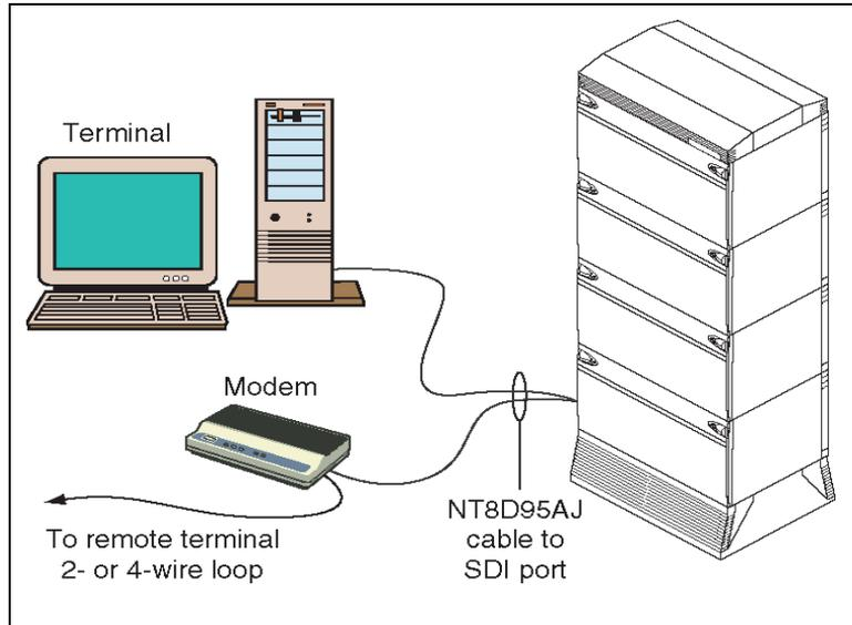
During the initial installation of a dual CPU system, you may want to temporarily install additional terminals for split mode monitoring, or programming, or both.
