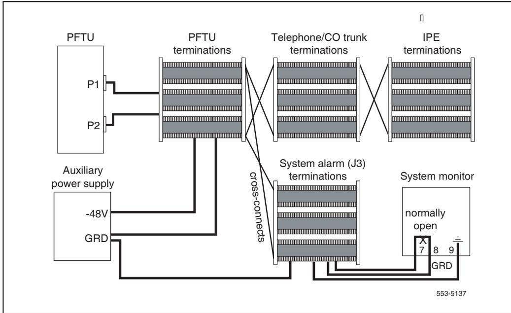
Figure 62 on [page 151](#) shows detail view of the PFTU alarm connections. The PFTU can be activated by system power failure and using the Attendant console TC switch. If more than one Attendant console is connected to the system, it must be connected in parallel with the main Attendant console as shown in the figure.
