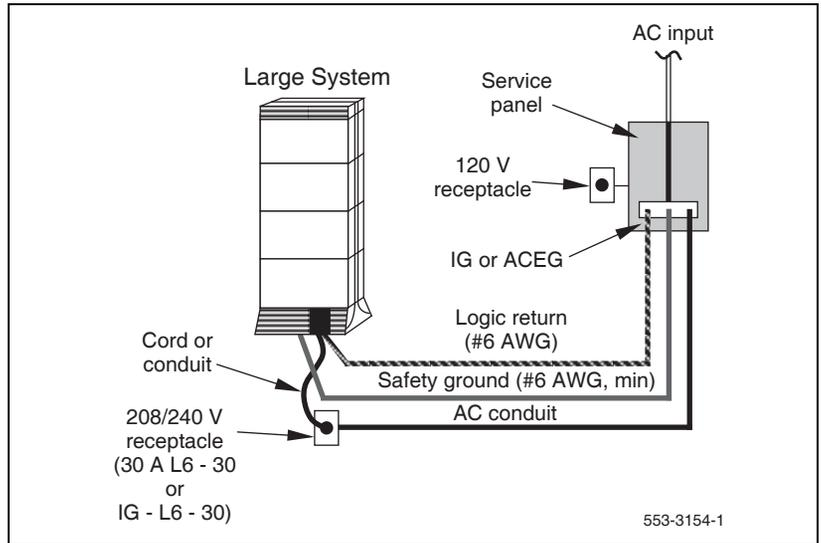
**Note:** In an isolated ground system, the dedicated isolated ground bus bar in the service panel serves as the ground window. It is used for all AC safety grounds and logic returns. It also accommodates a conductor that references the (+) battery bus in DC systems.
