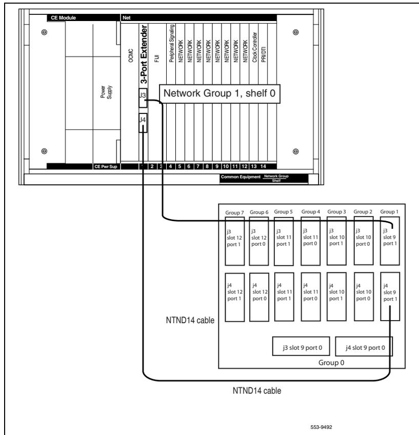
Refer to Table 62 on [page 376](#) for cCNI port and slot assignments. Connect Shelf 0 3PE cards to the Core/Net 0 panel; connect Shelf 1 3PE cards to the Core/Net 1 panel. The 3PE cables for Network Group 0 are factory installed.
