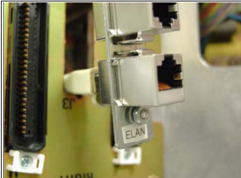
Figure 47 ELAN connection on Ethernet port coupler
