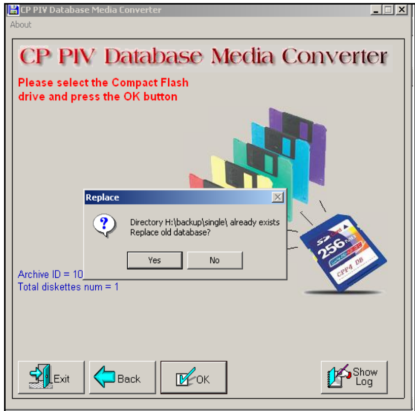
Figure 8 Replace database on CF drive
