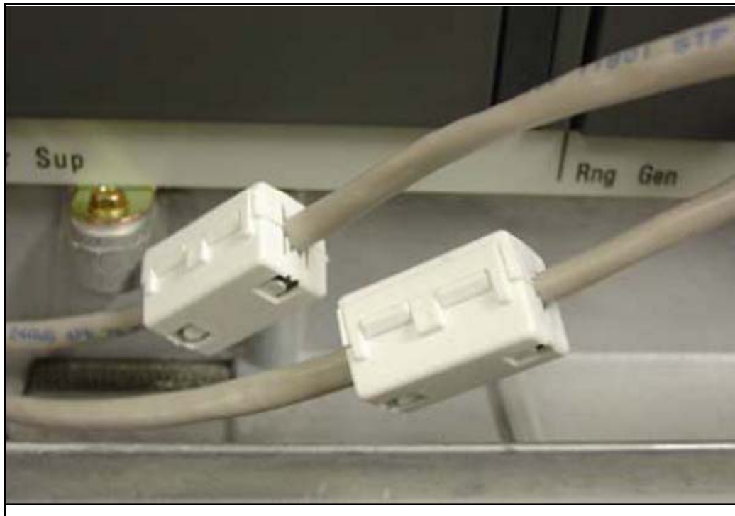
Figure 51 Attached Ethernet patch cable ferrite beads
