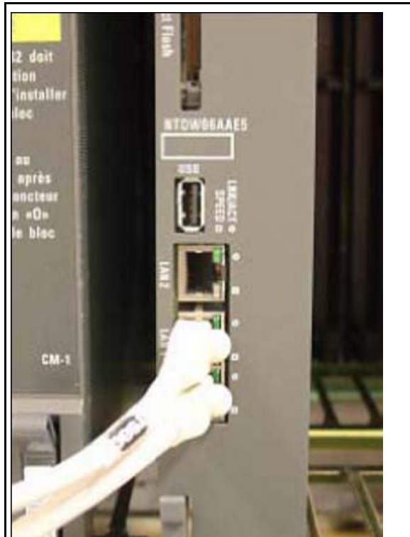
Figure 48 TLAN connection on CP PM faceplate
