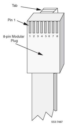
Figure 31: RJ-48-type 8-pin modular plug pin assignments
