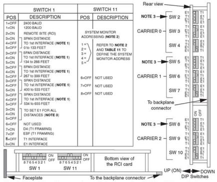
Note 1: SW1 switch positions 3, 4, and 5 specify the distance of each NT7R52AA Remote Carrier Interface card to the first signal regenarator, which can be a carrier repeater, a CSU, or an LTU.
