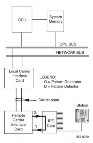
Figure 25: Loopback path for XCON test 7
