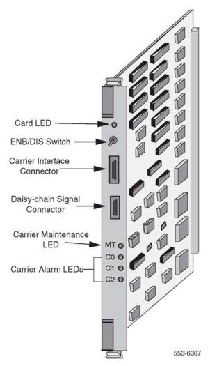
Figure 22: NT7R51 Local Carrier Interface card
