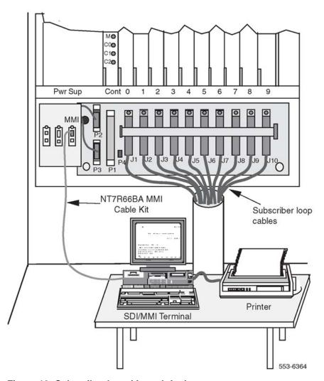
Figure 19: Subscriber loop (tip and ring) connectors
