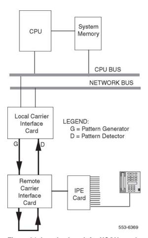
Figure 24: Loopback path for XCON test 6
