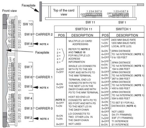
Note 1: SW1 switch positions 3, 4, and 5 specify the distance of each NT7R51AA Local Carrier Interface card to the first signal regenarator, such as a DNI, a repeater, a CSU (T1), or an LTU (E1).
