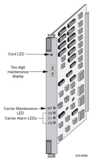
Figure 23: Remote Carrier Interface card
