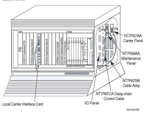
Figure 10: Local Carrier Interface card faceplate cable connections in Meridian 1 PBX 61C
