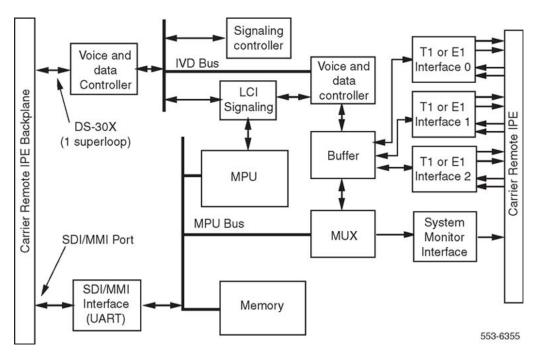
Figure 7: Remote Carrier Interface card functional block diagram
