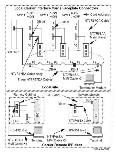
Figure 12: Daisy-chaining multiple Local Carrier Interface cards
