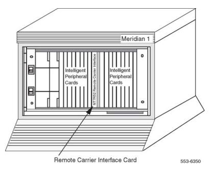
Figure 2: Carrier Remote IPE column
