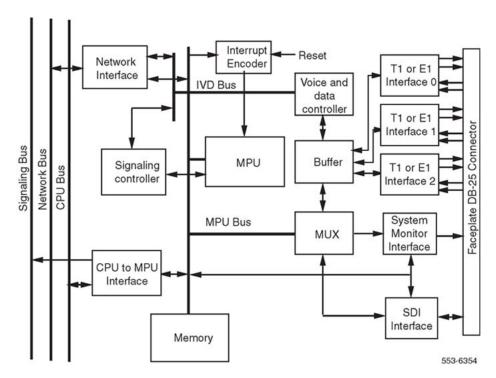
Figure 6: Local Carrier Interface card functional block diagram
