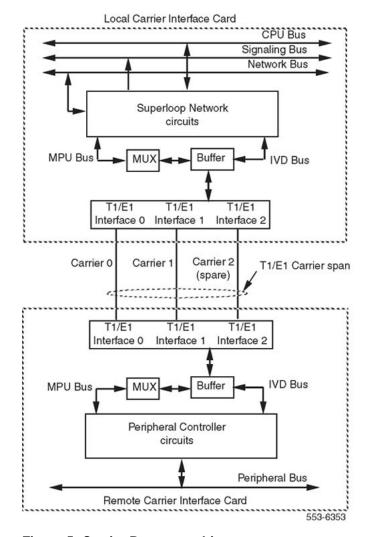
Figure 5: Carrier Remote architecture
